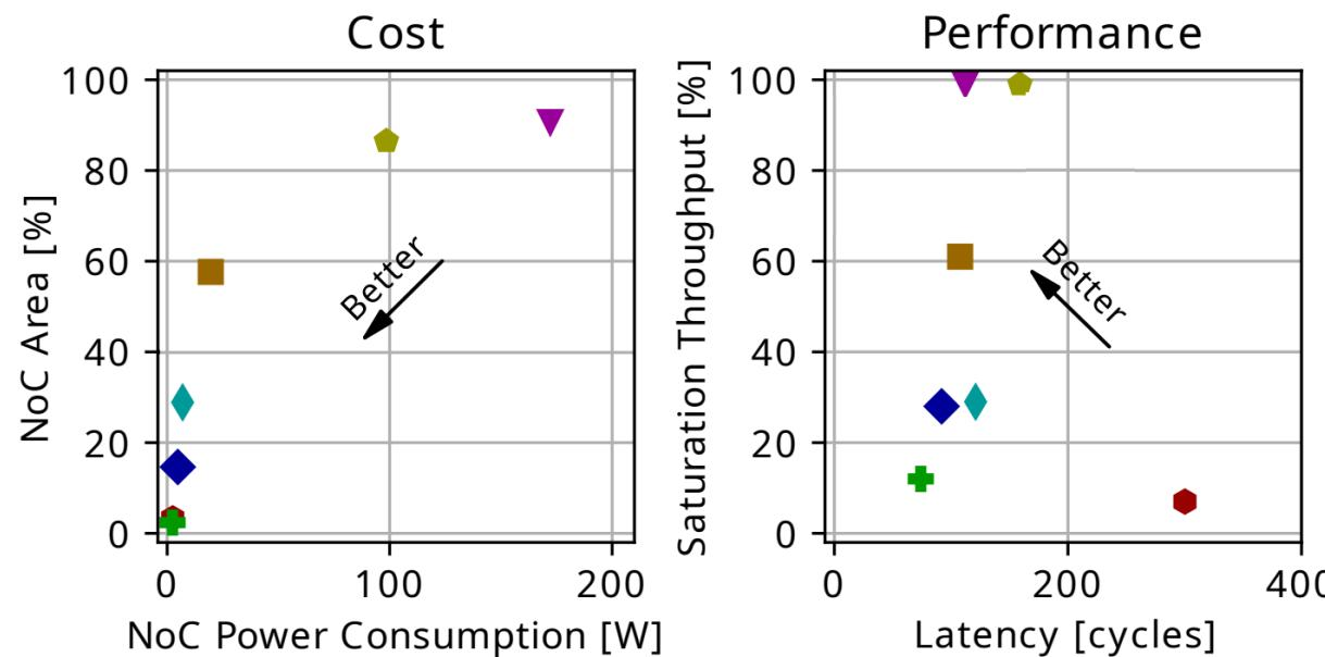
◆ Ring   + 2D Mesh   ♦ 2D Torus   ◆ Folded 2D Torus   ■ Hypercube   ▲ SlimNoC   ▼ Flattened Butterfly
