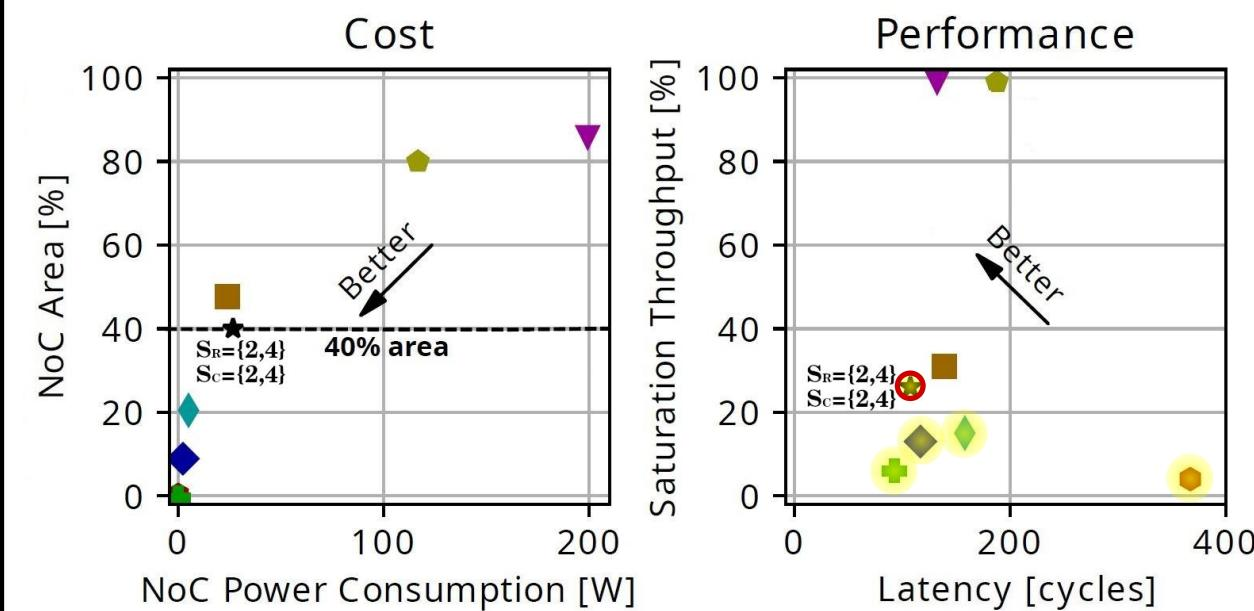
● Ring   + 2D Mesh   ◆ 2D Torus   ♦ Folded 2D Torus   ■ Hypercube   ▲ SlimNoC   ▼ Flattened Butterfly   ★ Sparse Hamming Graph (This Work)
