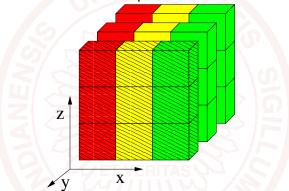
pattern means that data was transformed in y and z direction
